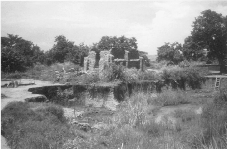
Figure 6. Tejera #524 with borrow pit in foreground, and kiln with workspace and drying blocks in background.
