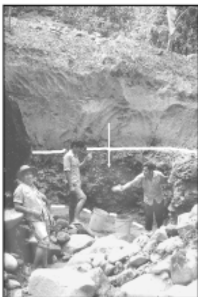
Fig. 4 (a,b): Placer mining operations at the Quebrada Barrera, Caribbean Veraguas, 1977: (a) A Ngöbé native American washes gravel looking for gold at a lavadero (photo by R. Cooke); (b) Extraction of fluvial gravel in a search for gold. The arrow points to the auriferous deposits, which are below the horizontal white line (photo by R. Cooke); (c) Raw materials for metalsmiths from Sitio Conte: 1. Copper bar found in Lothrop's grave 26; 2. Ingot, 89% gold, 11% copper, trace silver; 3–4. Ingots, 97.6% gold, 2.4% silver, apparently unprovenienced; 5. Ingot, composition not analyzed, Lothrop's trench II, general digging (based on Lothrop 1937: fig. 46).
